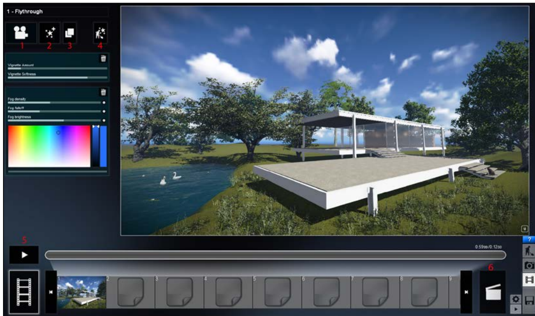
The Movie menu interface with the clip we just created: 1 - Edit clip, 2 - New effect, 3 - Copy, 4 - Build with effects, 5 - Play, 6 - Save movie
